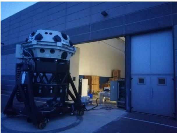
Figure 28. Flyeye telescope in Turate waiting for sky night observation.
