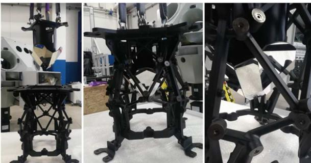
Figure 13. New aspherical lenses frame manufactured to solve mainly the upper channels obstruction.
