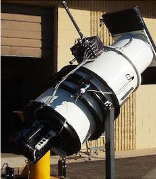
Figure 4. ATLAS 0.5-m F/2 OTA in its test stand at DFM Engineering (courtesy: DFM Eng.).
