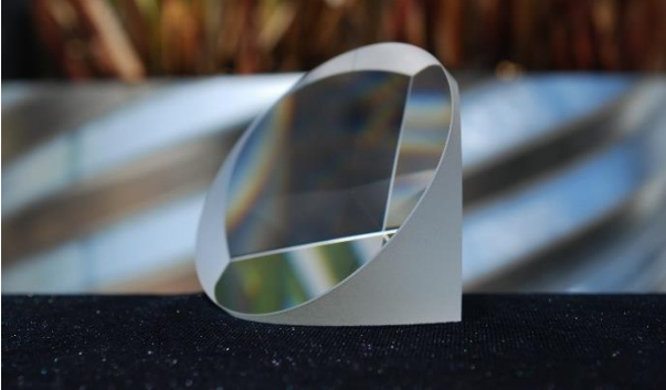
Figure 4. Example of a corner cube retroreflector. Credits: Precision Optical [4]
