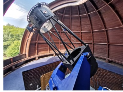
Figure 1. AGO70 newton telescope on fork equatorial mount inside of its dome at Astronomical and Geophysical observatory in Modra [2].
