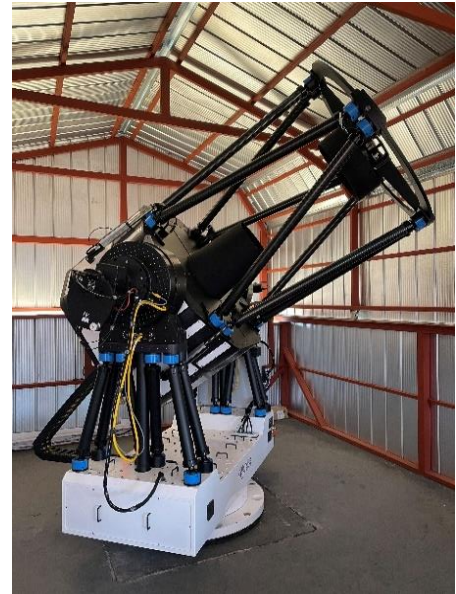
Figure 5. PAN 10 sensor (site: Deep Sky Chile, CDK1000, aperture: 1000 mm).
