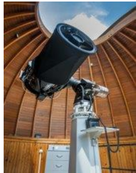
Figure 6. The SHOT sensor (site: Teplice, Czech Republic, CDK17, aperture: 432 mm).
