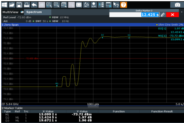
Figure 8 Received signal power from Cheia 2 as it is locked on Taurus (0.5 deg AZ step response)
