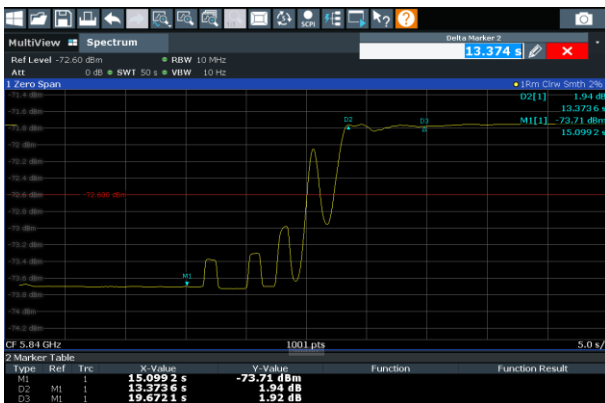
Figure 9 Received signal power from Cheia 2 as it is locked on Taurus (0.5 deg EL step response)
