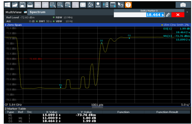
Figure 11 Received signal power from Cheia 2 as it is locked on Cassiopeia A (0.5 deg EL step response)
