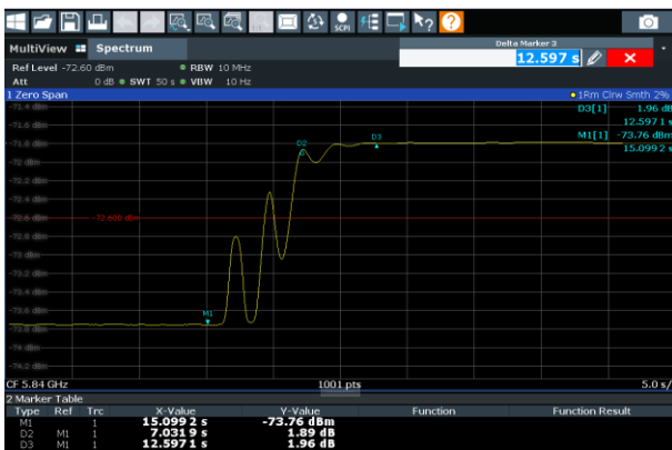
Figure 10 Received signal power from Cheia 2 as it is locked on Cassiopeia A (0.5 deg AZ step response)
