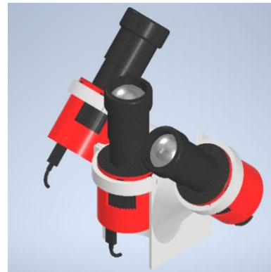
Figure 4: CAD model of the final LOCI camera mount design
