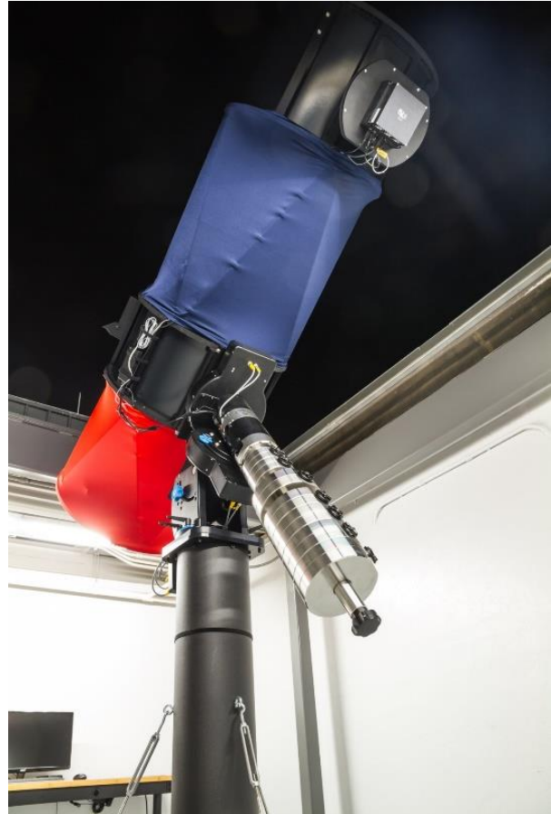
Figure 4. RAPTORS telescope for spectroscopic survey of GEO Belt.
