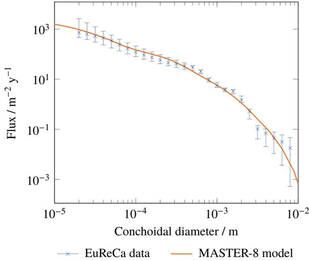
Figure 6: Comparison of simulated impacts based on the MASTER population with retrieved solar arrays from the European Retrievable Carrier (EuReCa).
