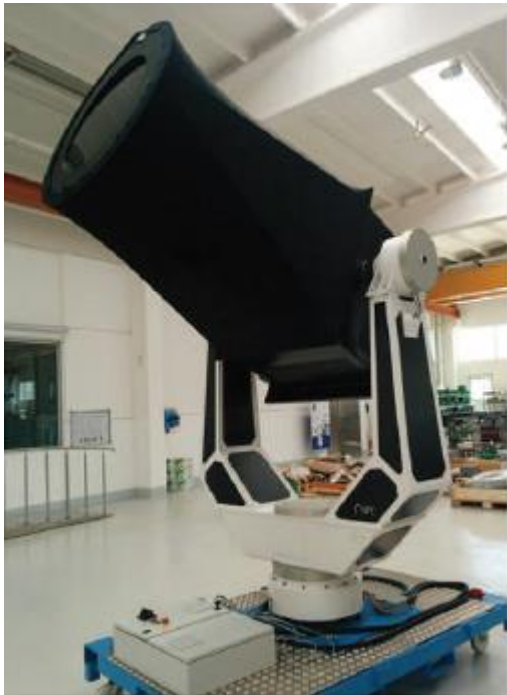
Figure 3. Moral M1000 with one meter class telescope mock-up for testing in relevant conditions
