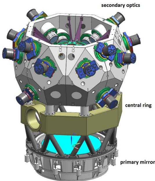
Figure 3. NEOSTEL Opto-mechanical Assembly
