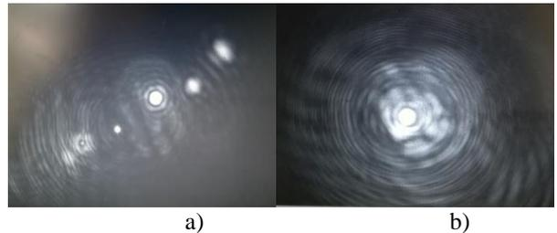
Figure 11. Newton's ring families generated by the optical channel components a) before and b) after alignment.
