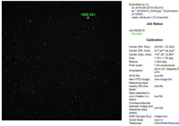
Figure 8. Example of a calibrated and astrometrically reduced image, as obtained by a 0.5s exposure at the factory observation site. It was possible to identify c.a. 2300 catalogued sources per optical channel.
