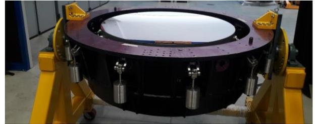
Figure 5. NEOSTEL Primary Mirror within Off-load System during Integration and Test
