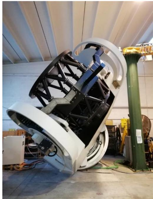
Figure 7. NEOSTEL Equatorial Mount at manufacturer's premises during acceptance tests
