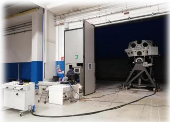
Figure 6. NEOSTEL mounted on a mechanical ground support, allowing two axes rotations, during night sky observation campaign at OHB Turate's premises.
