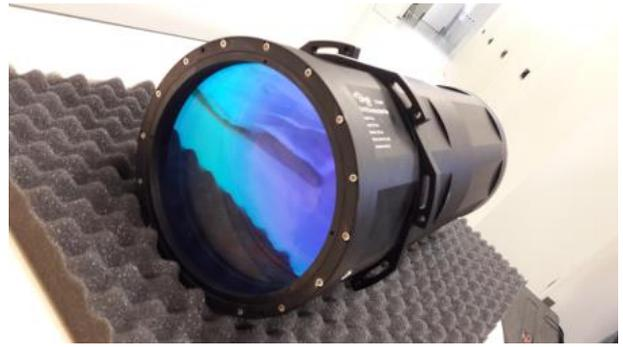
Figure 10. Secondary Optical Tube as seen from the pass band filter side.
