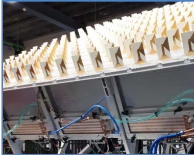
Figure 8. Partial view of a Rx Building Block (without radome) fully populated with reception modules.
