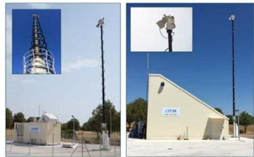
Figure 11. Tx antenna calibration (left side) and Rx antenna calibration (right side) setups
