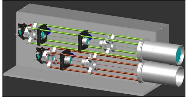
Figure 3. Laser package with two transmit telescopes
