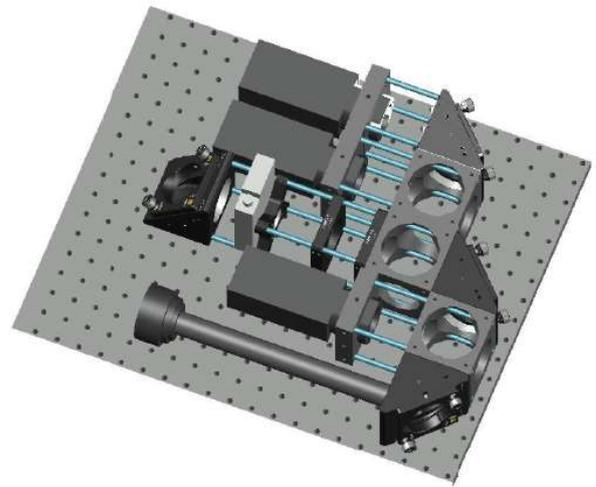
Figure 4. Detector package for two wavelengths, light curve detector (prepared) and tracking camera
