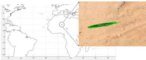
Figure 2. Footprint visualized on Google Earth of the fragments area of the D-SAT satellite during the in-space validation of the DeCAS system
