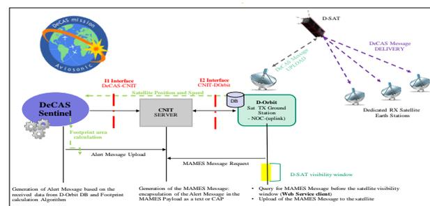
Figure 5. DeCAS in orbit concept demonstration mission architecture
