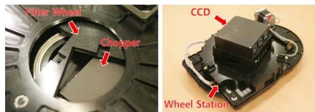
Figure 2. Detector Subsystem Hardware which is Composed of a CCD Camera, Filter Wheel, Chopper and Time Tagger
