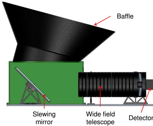
Figure 2. The concept of SODA telescope with slewing mirror.
