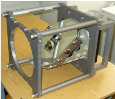
Figure 3. Slewing mirror for meteorological satellites Electro-L.
