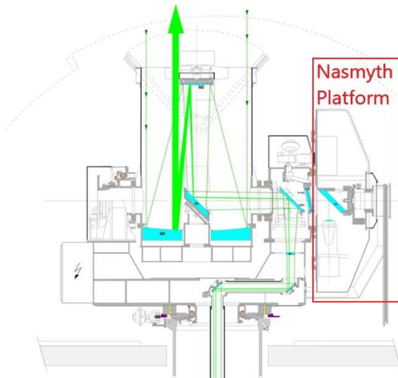
Figure 2 Sketch of ZIMLAT Telescope.
