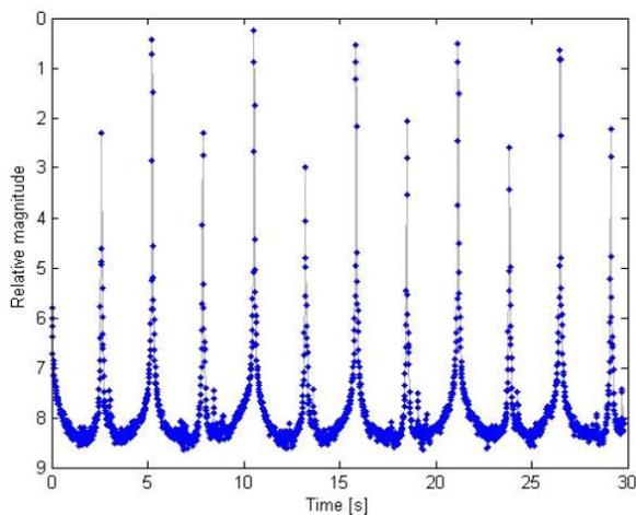
Figure 5 Light curve of N1 (78018B) rocket stage acquired by ZIMLAT.
