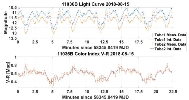
Figure 21 Extracted light curve and corresponding color index obtained for a Delta 4 rocket body (11036B) from ZimTWIN measurements.
