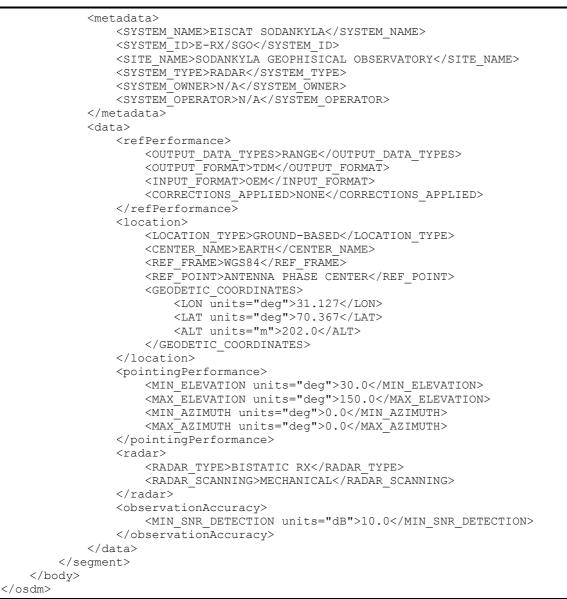
Figure 3 - Example OSDM in XML for a radar
