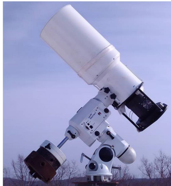
Figure 4. Typical 19.2-cm telescope VT-78a with field of view 7x7 degree for extended GEO survey in Ussuriysk (Far East)
