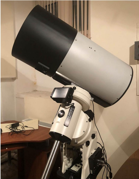
Figure 8. New 40-cm telescope SANTEL-400/500 with field of view 5.5x4 degree for asteroid survey that will be installed in Multa (Republic of Altai) in 2019
