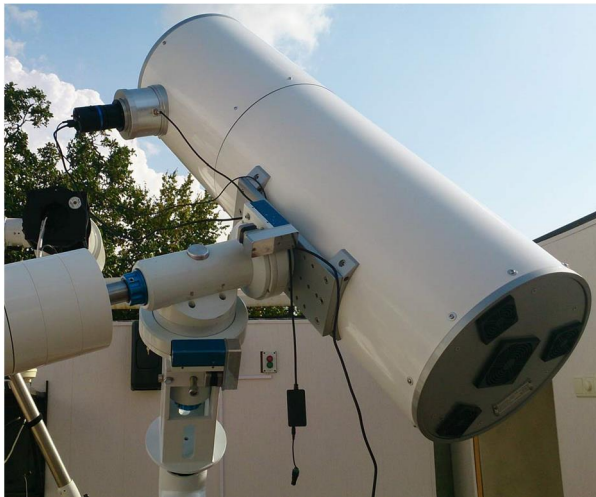
Figure 6. First 40-cm telescope DIN-400 with field of view 25x16 angular minutes for high precision measurements in Nauchny (Crimea)
