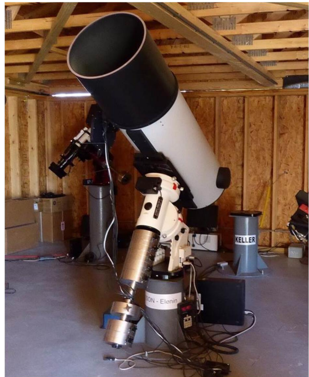
Figure 7. Old 40-cm telescope SANTEL-400A with field of view 1.65x1.65 degree for asteroid survey that worked in New Mexico (USA) during last 6 year
