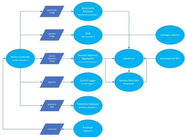
Figure 6. High-level station-cloud interaction.
