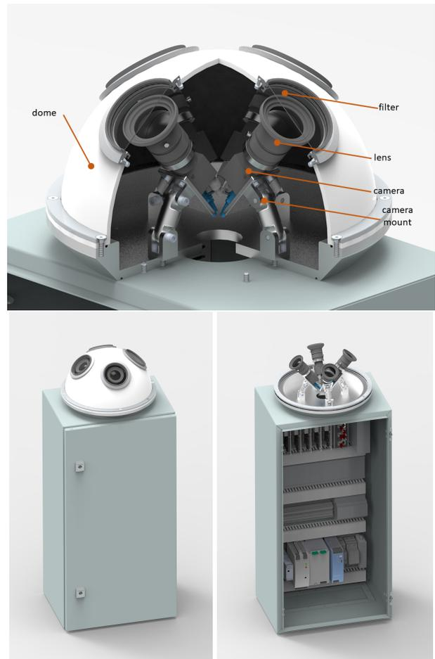
Figure 3. OmniSky station design renderings: dome details (left), full assembly (centre), interior (right)
