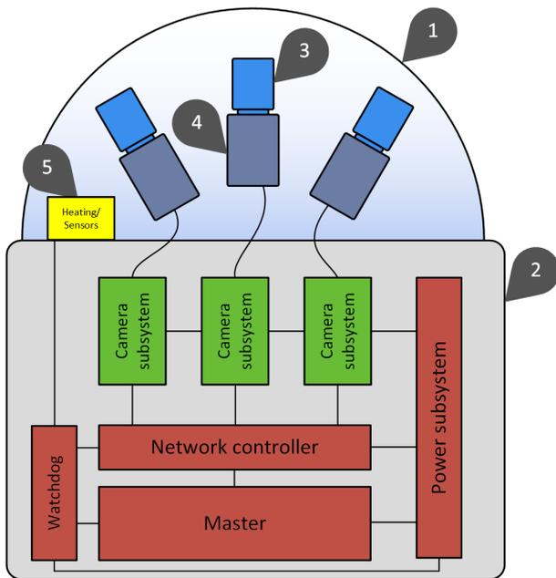
Figure 2. OmniSky station hardware architecture concept. 1 – camera and lens housing; 2 – electronics’ housing; 3 – camera lens; 4 – camera; 5 – heating/sensors module.
