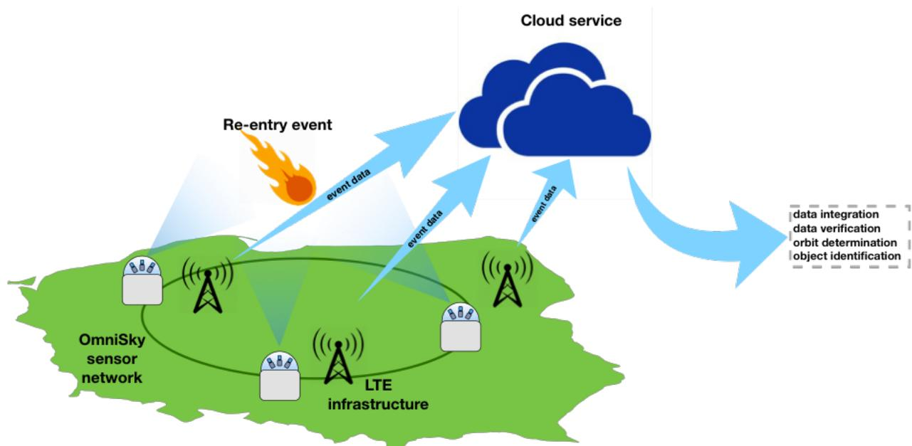
Figure 1. OmniSky concept. The sensors are designed so that they can operate on 3G networks. Data acquired by the stations is processed in real-time and potential re-entry events are transferred to the cloud for further computing and integration with data from other sensors.
