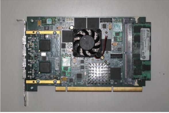
Figure 6. FPGA board developed for the algorithm
