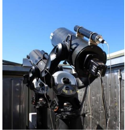
Figure 11. The remote observation site at the Siding Spring Observatory in Australia. 3 telescopes (two 25cm-telescopes and one 18cm-telescope) with the wide-field CCD cameras manufactured by FLI are installed.
