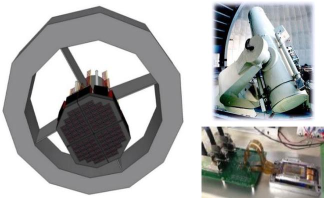
Figure 14. Tomo-e Gozen Camera (left). 84 chips of 35 mm full HD CMOS image sensors are installed at the focal plane of 105cm Schmidt telescope at the Kiso observatory (upper right). The lower right shows the readout electronics of the Tomo-e Gozen Camera.
