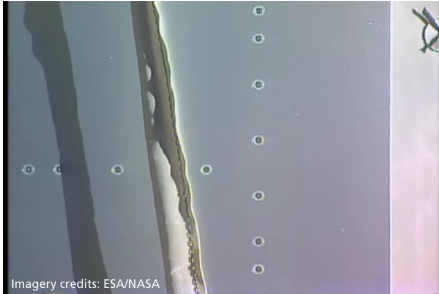
Impact craters on the surface of the Columbus module
