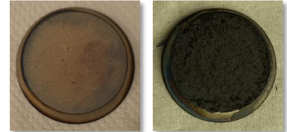
(oxidised in IRS PWK1 facility at LHF-1 test condition at varying exposure times [Pagan2016, Pagan2015])
