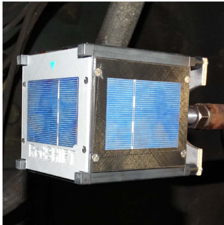
sample set up in the wind tunnel
