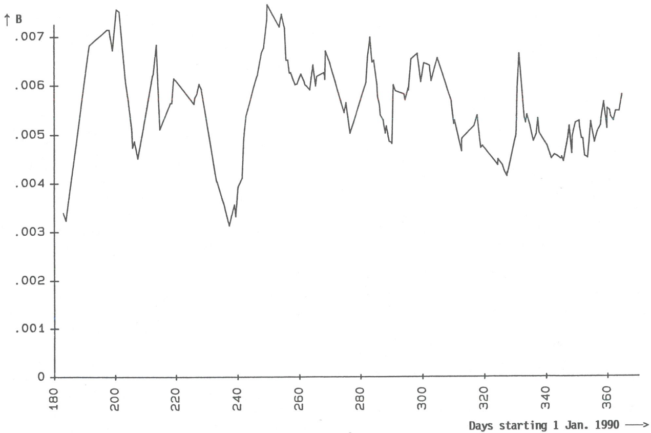
Fig. 4.1: Determination of the ballistic coefficient B (m 2 /kg), value averaged over three 27-days solar rotation cycles.
